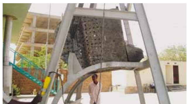
The guide rails of the HUBER CageLift are curved in the upper discharge area, so that the filled screen basket can be moved directly over a container and emptied semi-automatically.
