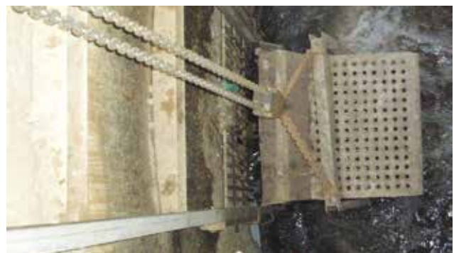
Reliable and safe guidance of the screen basket by means of guide rails arranged on both sides.
