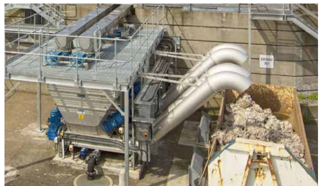
Well washed and virtually odorless screenings from a HUBER Screenings Wash Press WAP® SL, compacted to 50 % DS.
