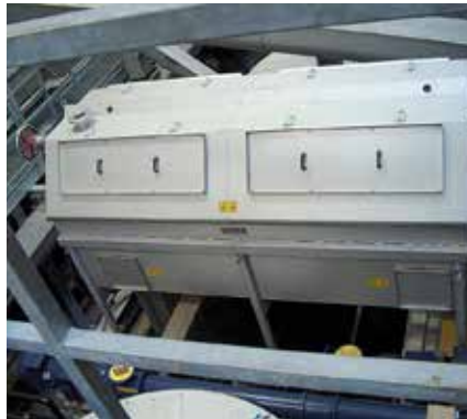
HUBER Drum Screen RoMesh® screen for the removal of fine and finest particles.
