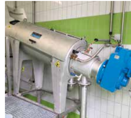
HUBER Screw Press Q-PRESS® for surplus sludge dewatering in mineral water / mixed beverage industry.
