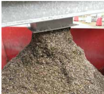
Plastics separated by fermentation residue screening.
