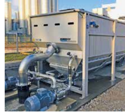
Flotation plant HDF S for high solids loads.
