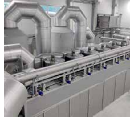
Sludge drying in industry with the HUBER Belt Dryer BT.
