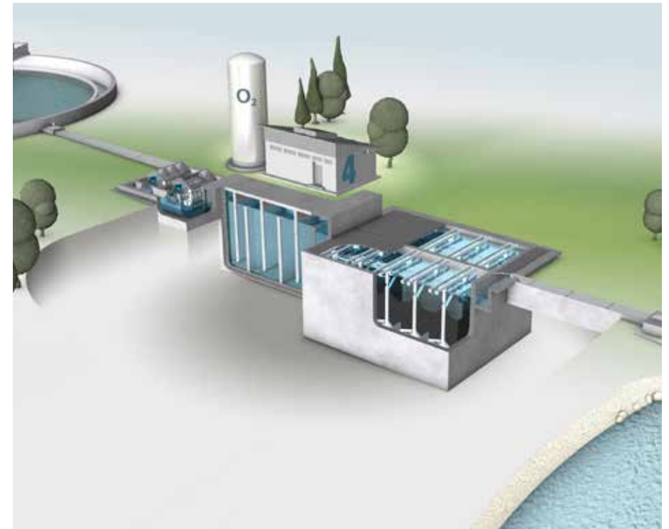
Advanced wastewater treatment for removal of trace substances with the combined process of ozonation and downstream HUBER Activated Carbon Filter CONTIFLOW® GAK.
