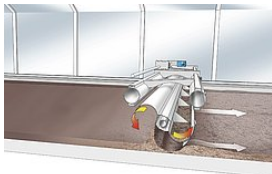
As the turning device travels forward, the sludge is being transported.
