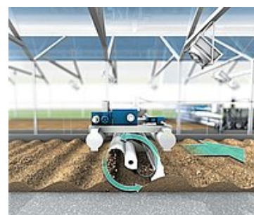
A double shovel is ploughing through the sludge bed and turning the sludge as the machine is moving through the greenhouse
