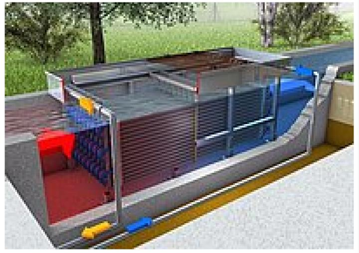
Recovery of heat from clarified wastewater provides several advantages: Considerable heat potentials are available due to the huge water volumes, effluent cooling does not have negative effects on the receiving water, and sewage treatment plants often have a high demand for heat.
